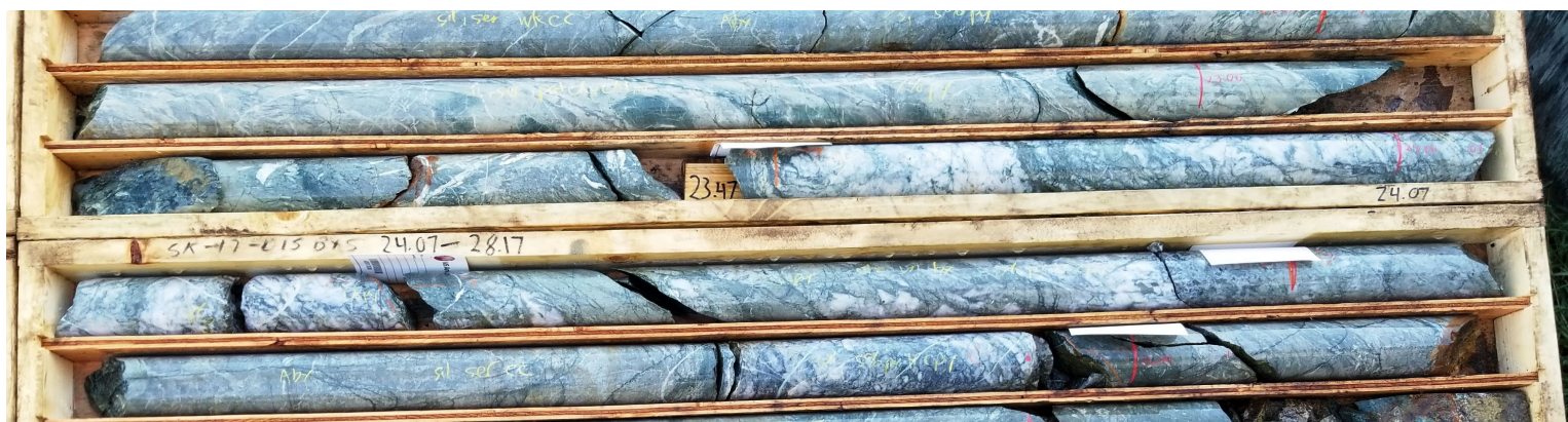
2017 Core from Swift Target – 2.5m (downhole) of 11.5g/t Au @ 23.5m in SQ17-015
